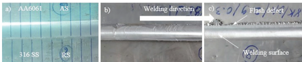
Fig. 4. Welding surface of the joint by different pin lengths: (a) 2.7 mm, (b) 2.8 mm, (c) 2.9 mm.
