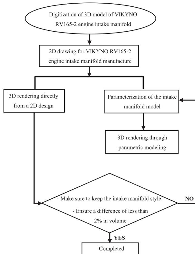
**Fig2.The process of performing 3D modeling of VIKYNO RV165-2 engine intake manifold by the parametric method.**
