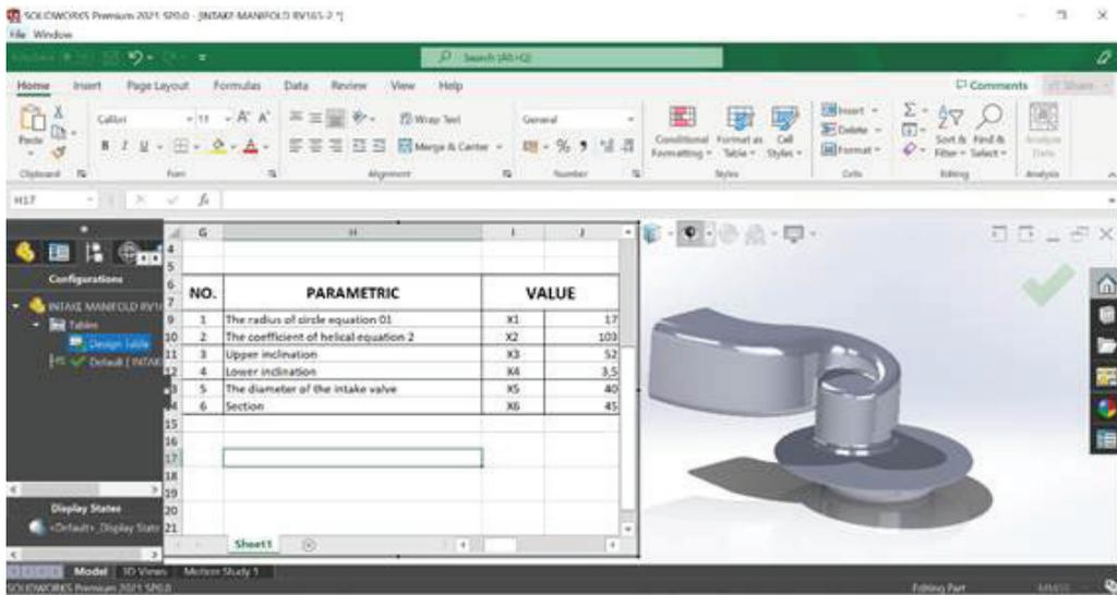
Fig. 7 Intake manifold rendered by the parametric method
