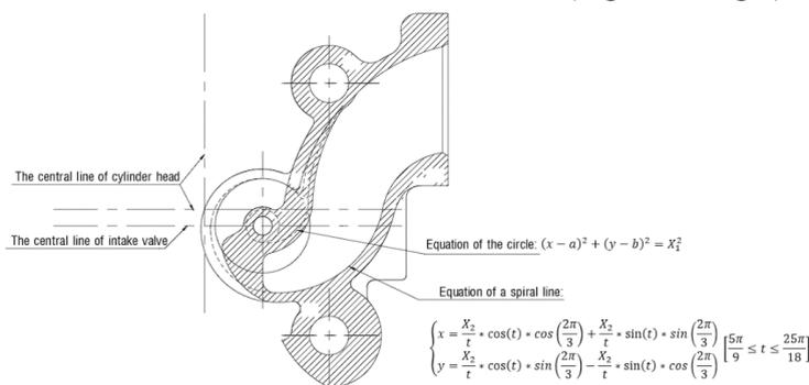
Fig. 5 The functions representing generatrices of the intake manifold.
