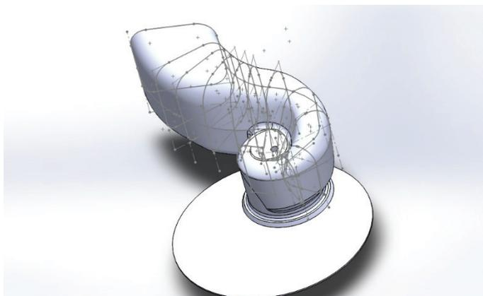
Fig. 4 Intake manifold rendered by 2D rendering method.
