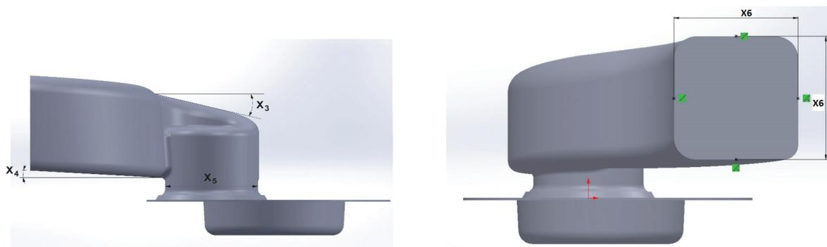
Fig. 5 The important geometric dimensions are chosen for parameterization.
