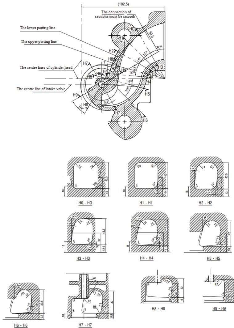
Fig. 1. Design of 2D intake manifold of Vikyno RV165-2 Diesel engine [7].
